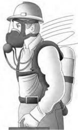
Self-contained breathing apparatus (SCBA) Pressure-demand mode APF = 10,000 Needs to be fit tested
